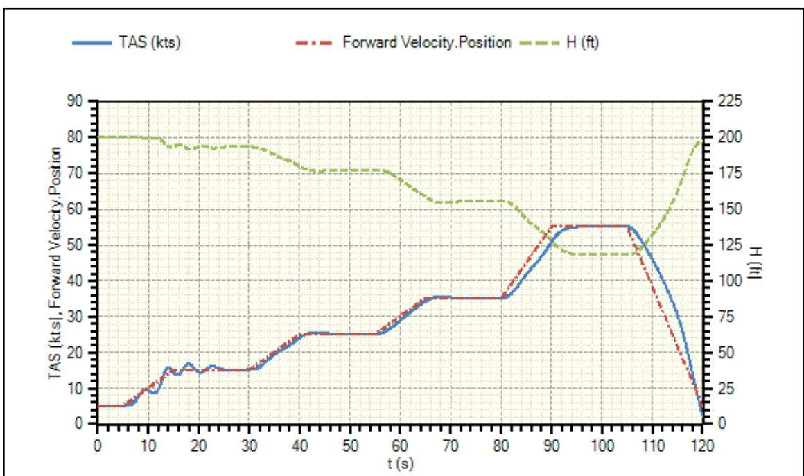
The response shows that using the target velocity to schedule the Pitch Control, Throttle, and Thrust Angle so the speed can be changed and the aircraft maintains stable flight.
