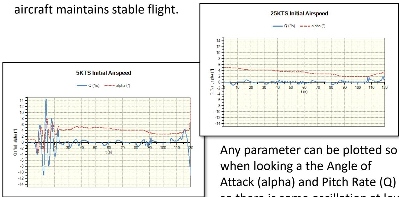
Any parameter can be plotted so when looking at the Angle of Attack (alpha) and Pitch Rate (Q) so there is some oscillation at low speed but at the higher speeds the aircraft is very stable.
