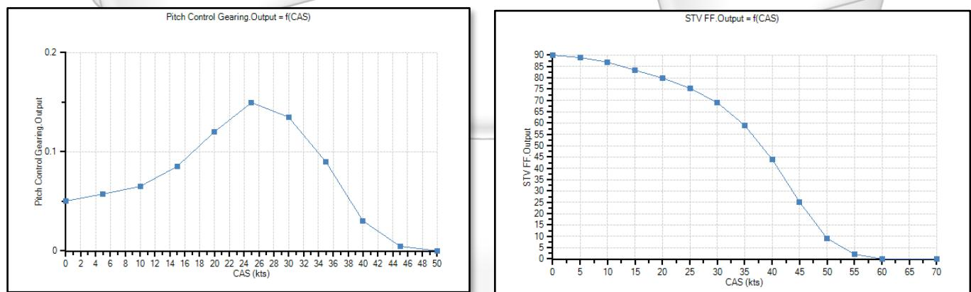
Response is evaluated and the scheduling adjusted to get the target behaviour. Due to the built in configuration management and version control the cases are re-run and the results assigned to a version number.
